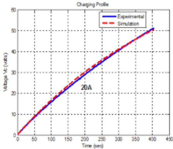
**Figure 3: Charging profile of BMOD0165 Super capacitor**
