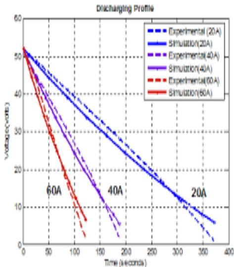
**Figure 4: Discharging profile of Super capacitor**
