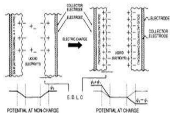
Figure 1: Super capacitor structure with positive and negative ions
